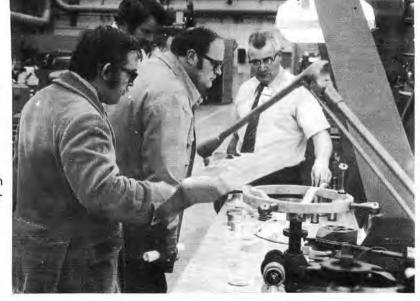
"variable pitch threads can be made only on a tape controlled lathe"
